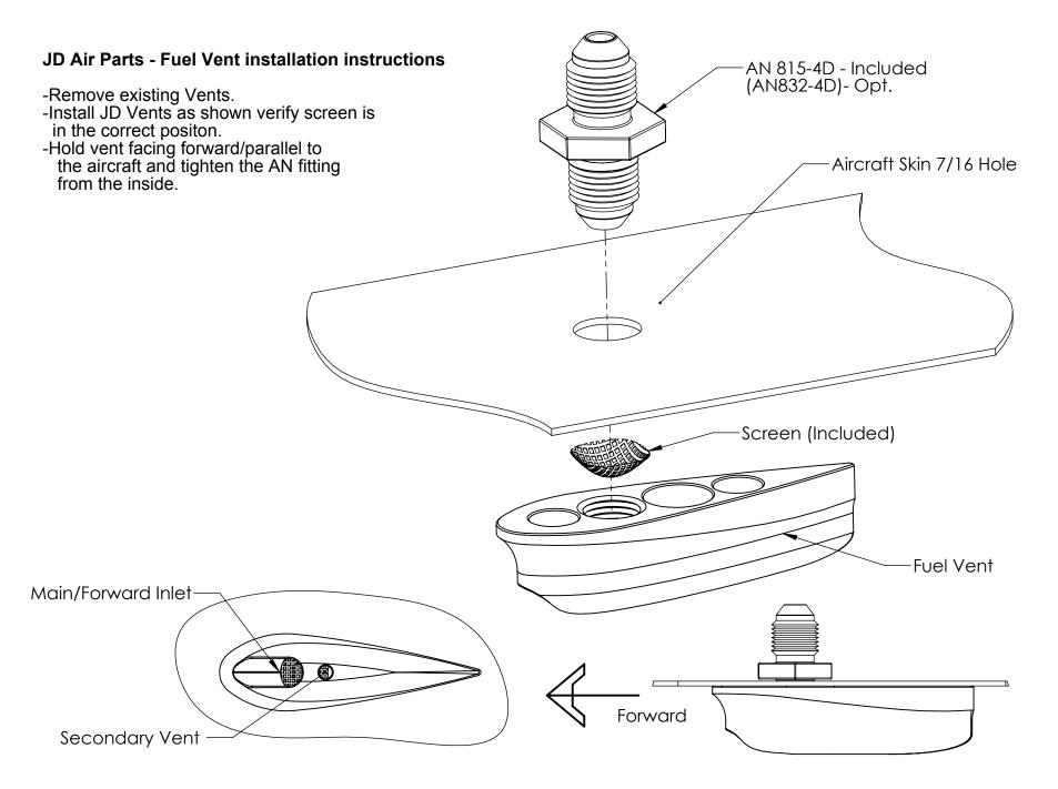
The JD Air Parts Fuel Vents have been tested to provide positive pressure and should NOT be operated in icing conditions. The secondary vent hole is provided to allow air flow to the tank if the forward inlet becomes clogged by debris.
