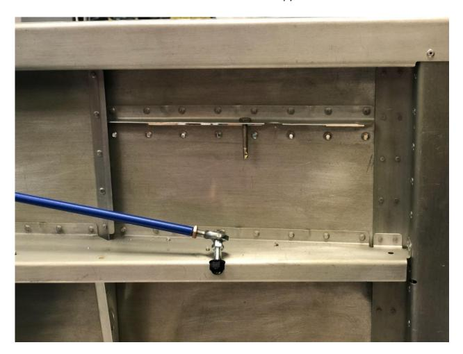
Mark the opening with the scaled template. The top can be trimmed at the longeron line. Tape the template to the side of the fuselage and trace inside of it after removing cut outs with razor blade.
