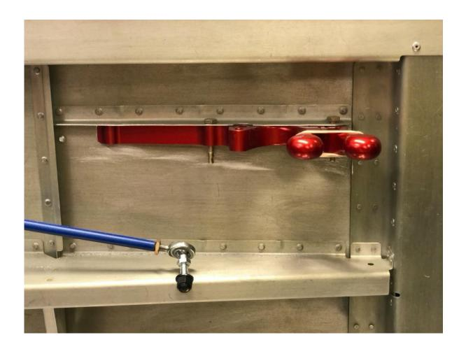
As you can see below, the spare rivet between the latches will hit the main latch. File/sand this down the best that you can without harming the structural integrity of the rivet, then counter sink a hole in the latch so it will fit flush.
